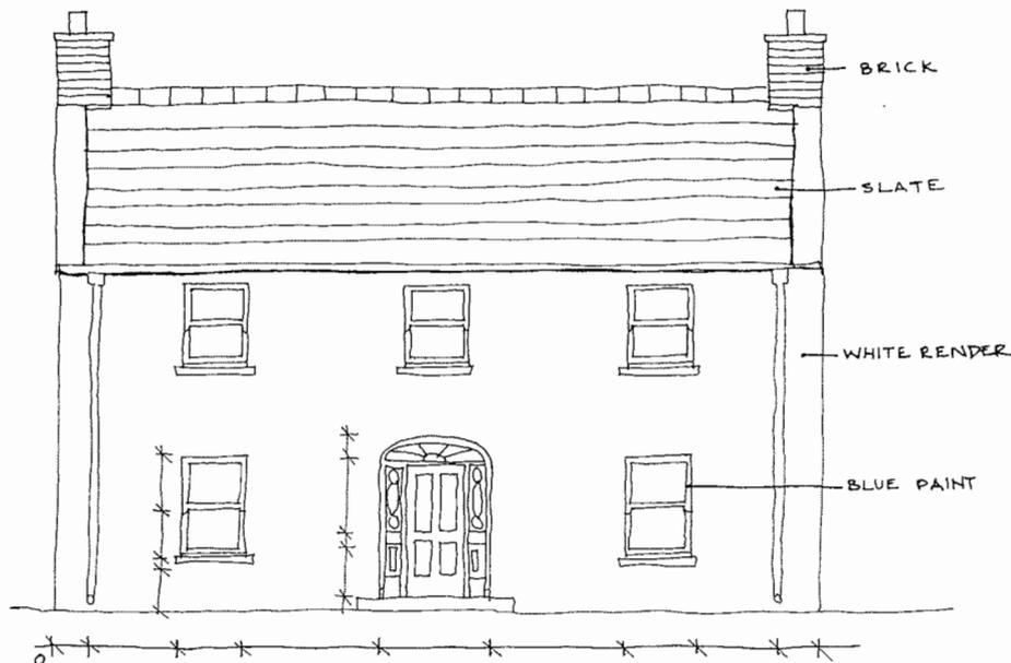
It is usually easy enough to measure the parts of the building near the ground. Take **horizontal measurements** along each wall just above the window sills. Note where windows, doors and any other features start and finish. Measure right around the building, starting at zero at each corner. Then take **vertical measurements** as high as you can reach from the ground. As you go along, note all of your measurements on the sketches you have made.
